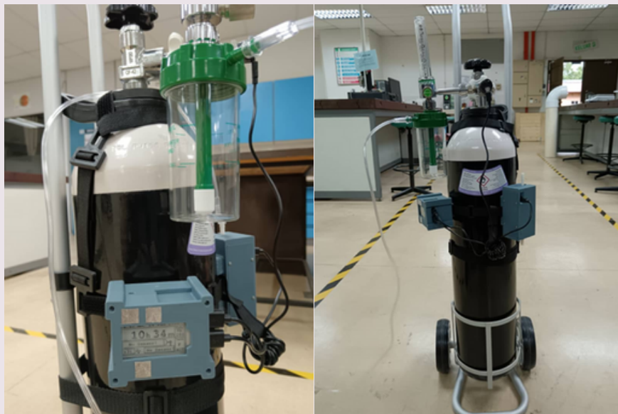
Figure 2: Final setup of SMOTMD applied to a typical oxygen tank.
